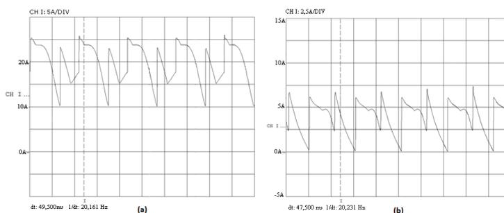
Fig. 6 Experimental waveforms of the current  $i_d$ : (a) for  $R_L = 30\Omega$ ; (b) for  $R_L = 100\Omega$
