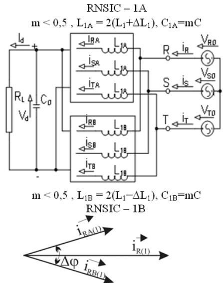
Fig. 3 Configuration of asymmetric RNSIC
