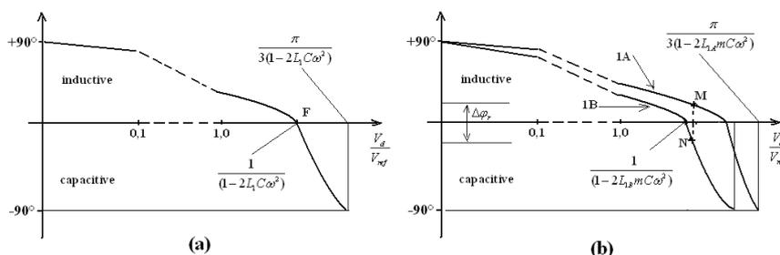
Fig. 4 Angle  $\varphi$  as a function of ratio  $V_d/V_{ref}$ ;
