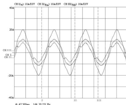
Fig.5 Experimental waveforms of the phase current  $i_R$  and the partial currents  $i_{RA}$ ,  $i_{RB}$ .
