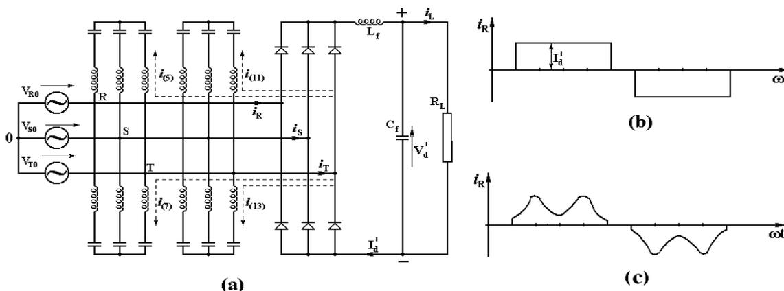
**Fig.1** Three-phase six-pulse full bridge diode rectifier with passive filters,
